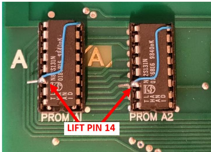
Connect pin 14 and pin 8 (GND) with a wire as in the picture. Both PROMs.
