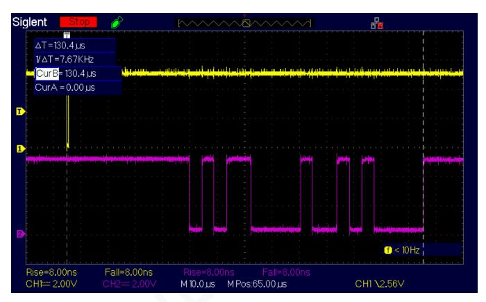
Total interrupt handling time and process time, added to serial transmission at 230400 baud: 130.4 µs
