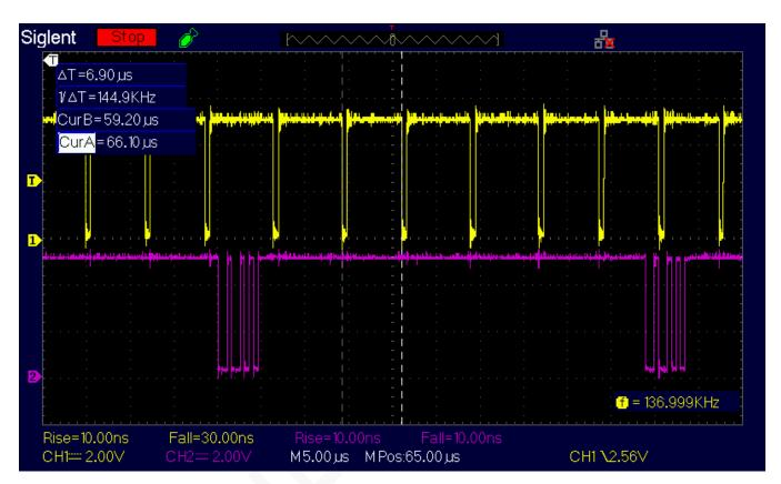
Overlap between interrupt signals and serial transmission at 2000000 Baud: loss of characters.
