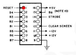
The red dot marks pin number 1. On the computer's motherboard and on the adapter the
