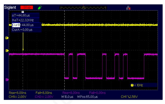
Microcontroller interrupt handling plus processing time, before starting transmission at 230400 baud: ~45 µs
