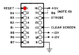
The red dot marks pin number 1. On the computer's motherboard and on the adapter the pin 1 is marked with a white dot.
