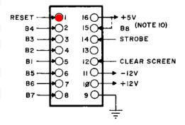
The red dot marks pin number 1. On the computer's motherboard and on the adapter the pin 1 is marked with a white dot.
